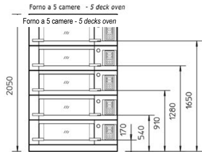
Forno con cella o basamento carenato (ruote optional) Oven with perfor or base-box (castors optional)
